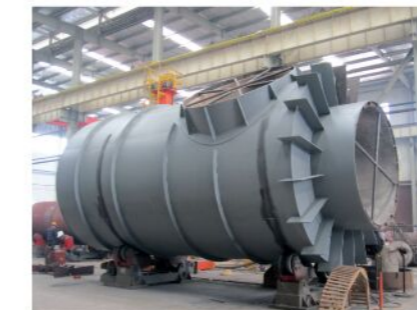
新型低压降水封罐 New model low pressure drop water sealed tank
