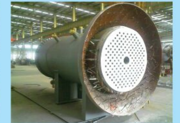
废热锅炉 Waste heat boiler
