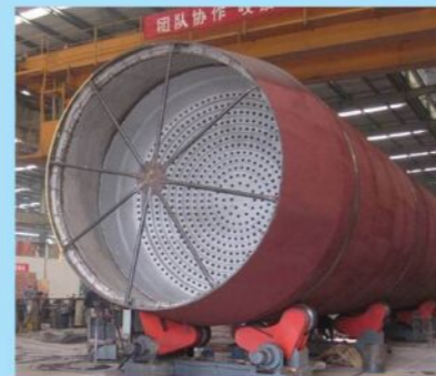
应用RT耐磨陶瓷喷嘴的降压孔板 Decompression orifice plate which equipped with RT anti-wear ceramic nozzle
